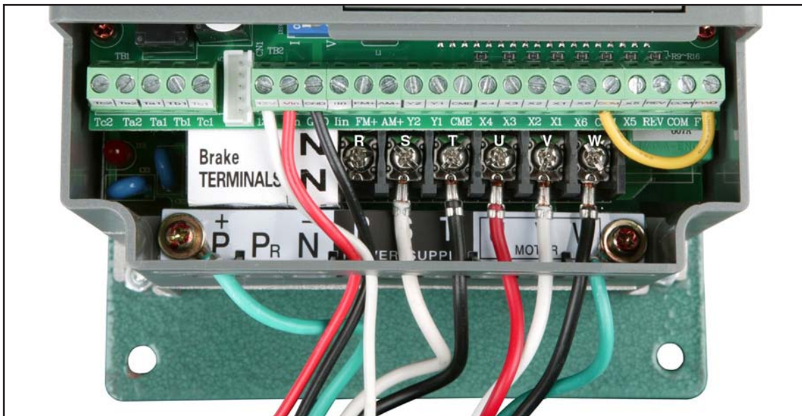
Figure 57. Inverter/controller box terminal blocks.
